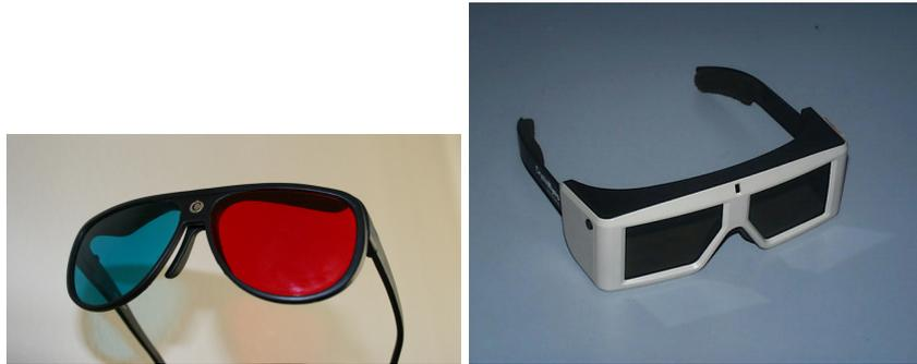
Figure 2.1: **Left image:** Glasses with anaglyph filters. **Right image:** LCD shutter glasses.
